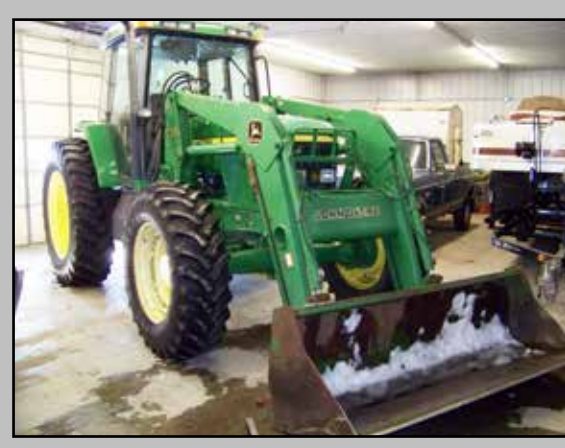
2000 John Deere 7510 Diesel Frnt whl assist, 2500 hours w/ JD 740 loader w/ bucket, 18.4-34 rears 14.9-R28 frnts all like new, 3 pt, PTO 2 hyd outputs
