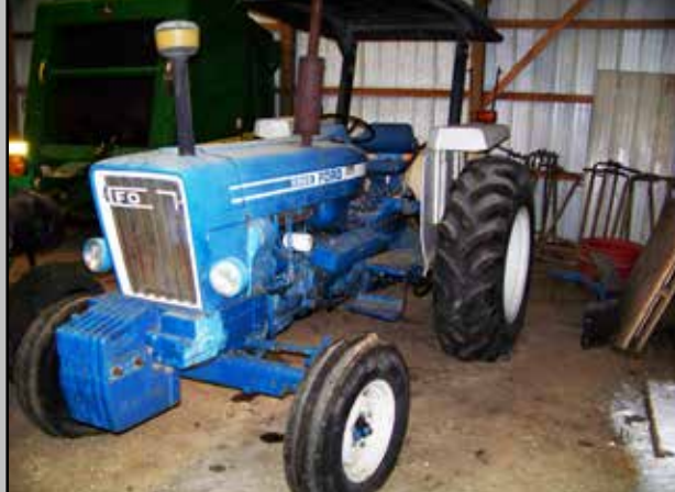
1988 Ford 5900 WF diesel, ser #ZX01449, 16.9-30 rears 50%, 1 hyd outlet, 540 PTO, drawbar, 2764 hrs, 6 suitcase weights, 3 pt.
