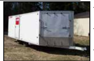
all aluminum enclosed 20' snowmobile trailer- front and rear ramp doors, side entry door, tie downs torflex axles.
