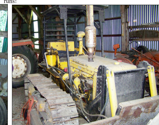
IH TD 9 Industrial crawler/dozer, 1951 mode, non running, Hyd 2 way blade, Diesel, 60% running gear, ser # TDCB41625
