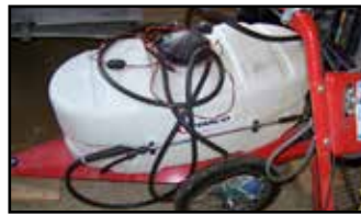
Fimco 20 gal portable sprayer, trlr mnt or ATV rack mnt, 12 v elec motor
