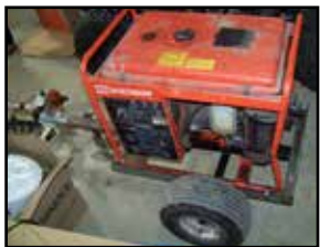
Multiquip 3k watt 208v 3 phase or 120v portable gas generator on utility cart.
