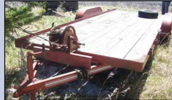
20' tandem axle 7000 lb car trailer w/ hand crank winch
