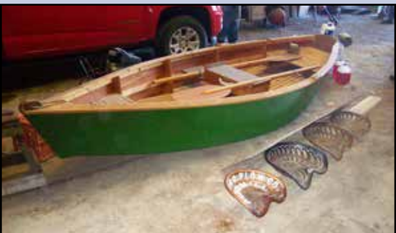
Western style 14' river boat, slatted floors, highly rockered, said to have been built in Erskine, appears to be new and of a high quality build
