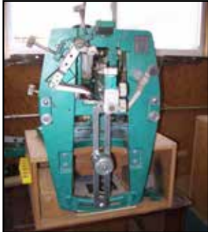
Foley Belsaw mod 357 circle saw carbide blade grinder
