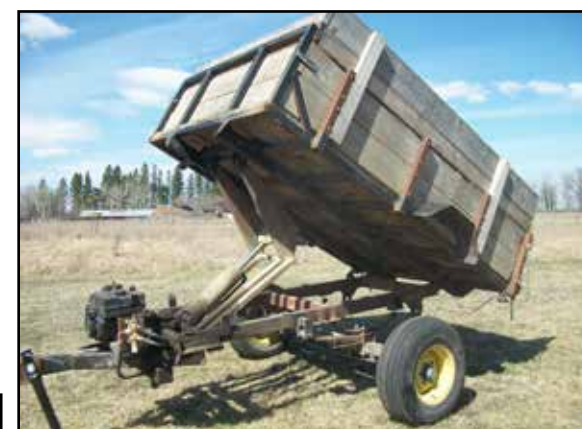
Shop Built single axle 6'X9' hydraulic dump trailer w/gas engine for Hydraulics works great
