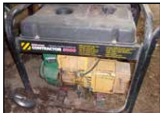
5kw contractor generator
