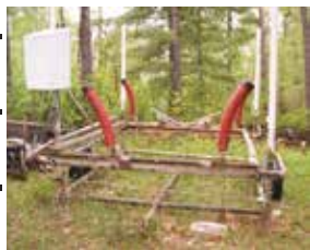
Cantilevered electric boat lift w/ canopy
