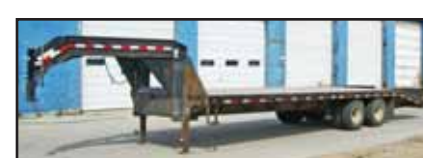
24,000lb Goose neck trailer w/tandem dually's, 8X22 wood bed w/6' Beavertail. Dual landing gear, front service box, good rubber DOT'd in '11.
