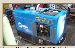
Like new Miller Bobcat 250 NT Welder-Generator 20 hp 250 Amp 10k watt CC/CV AC/DC stick welder and Miller SGA 100c spool gun control and cart (adds wire feed capability to the welder)
