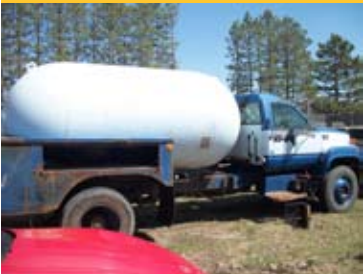
'97 GMC 7500 propane delivery truck, 103K mi on odometer, 3116 CAT Diesel 6 speed manual, DOT'd 2010 lic Feb '12, w/ Arrow 2500 gal propane tank, Liquid controls pump & printer w/hose reel
