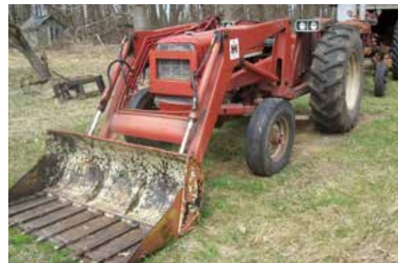
IH 574 gas tractor WF W/IH loader, 3 pt 16.9-30 rears ser # 2310076U107898 4spd w/ Hi/Lo range, 1 hyd, 540 PTO, 2687 hrs
