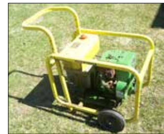
John Deere 3500 watt generator
